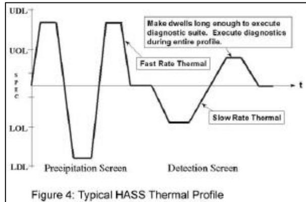
used. A baseline for the stresses is derived by guardbanding the limits found in HALT. Typically, vibration is reduced by 50% and thermal excursions are reduced by 20%.<sup>1,2</sup> These limits can be used as a starting point for the Proof of Screen process.
